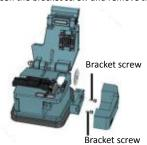
3.Put back the blade and holder, tighten bracket screw, then put back the side panel and tighten side panel screws.
