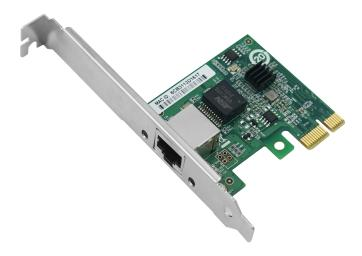
LRES2031PT is a PCle x1 single port 2.5G Ethernet network adapter developed by Elfcam, based on Intel master control scheme. This adapter provides better
