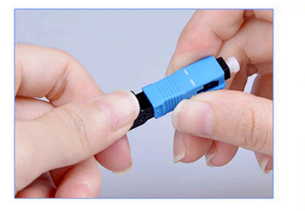
Put on the blue protective sleeve the assembly is complete
