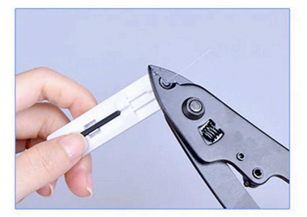
Use Fiber Optic Stripper Strip the fiber coating
