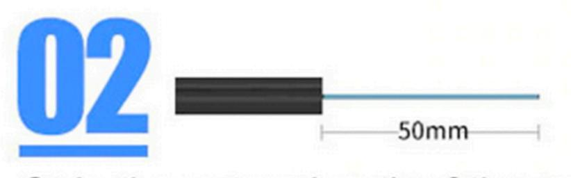
Strip the outer sheath of the optical cable and keep the covering layer. The length is 50mm.
